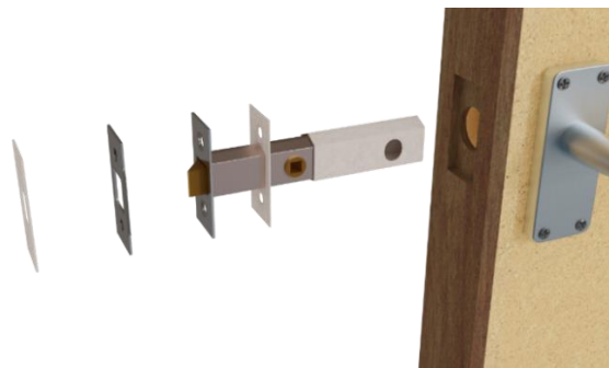
Example of lock & latch protection detail
