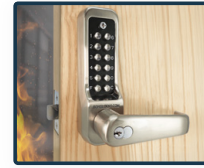
BL5401 ECP FT - Single sided keypad w/ 60mm tubular latch and key override – 60mm tubular latch •Satin Chrome •Satin Stainless
